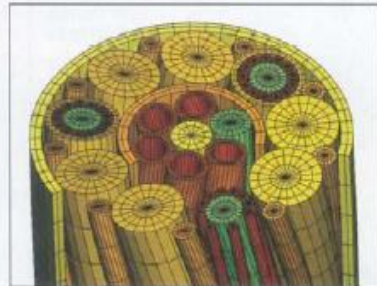
A cut-away view of meshed umbilical components. (Images courtesy of DeepSea Engineering)
