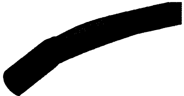
Figure 8: Collapse shape of carrier – design external pressure, bending moment increased until collapse
