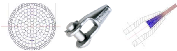
Figure 8 General Configuration; Left to right, Rope Cross Section, Conventional Socket Modified End Termination
